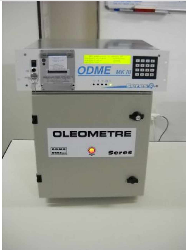
Figure 1: Fully Refurbished Seres MK-III Calculator with Darlas GPS Option and Oleo meter in full compliance with MEPC108(49).
